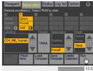
Figure 6.7: The separation program “Possel” will be performed on sample positions 1 and 2. After processing sample 2 the “Sleep” program will be performed as a final wash step before the instrument goes into sleep mode. Clicking “Run” will start the experiment.
