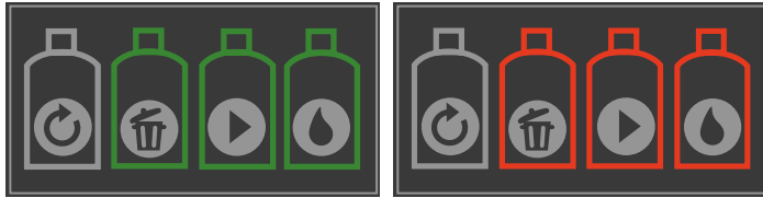
Figure 2.5: Left: Fluid bottles are shown in green indicating ready. Right: Fluid bottles are shown in red and need to be replaced.
