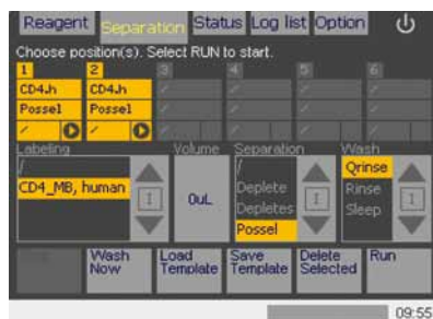
Figure 6.2: The Cell Separation Reagent CD4 MicroBeads, human was assigned to rack positions 1 and 2. The separation program “Possel” and wash program “Qrinse” were automatically selected.
