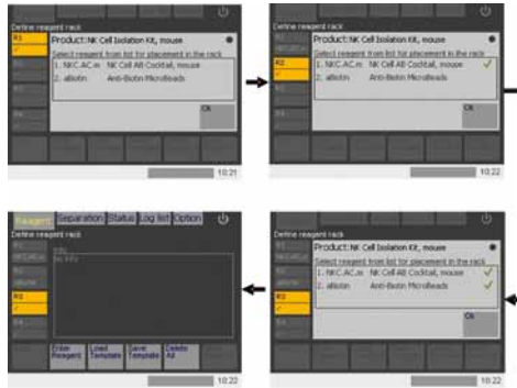
Figure 5.6: Entry of the components of the NK Cell Isolation Kit II, mouse . The reagent NK Cell Biotin-Antibody Cocktail, mouse was assigned to rack position "R1". The reagent Anti-Biotin MicroBeads was assigned to rack position "R2".
