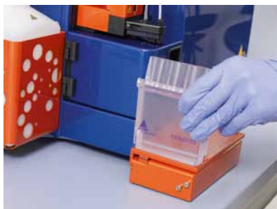
Figure 5.1: The MACS Reagent Rack 4 snaps into position as illustrated above.
